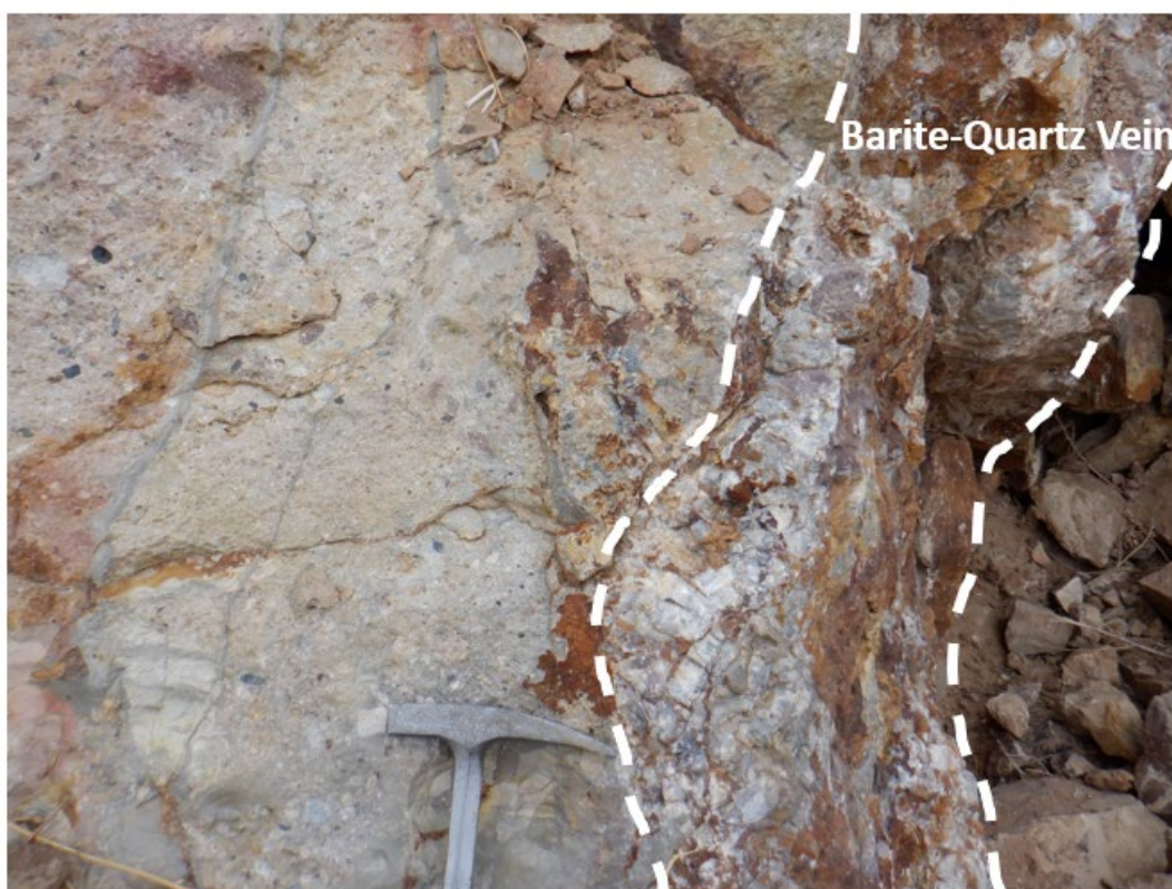
Photo 7.6 A general view of quartz-barite veins in Pickhandle formation, Langtry Project.
