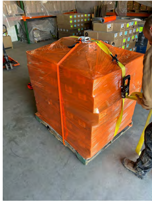
A pallet stacked with cardboard boxes of pulp samples is wrapped in translucent orange plastic shipping wrap, and strapped with two ratchet straps perpendicular to each other for stability.
