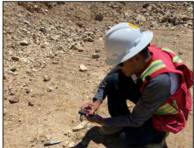
Drill Hole Location* Verification with GPS
